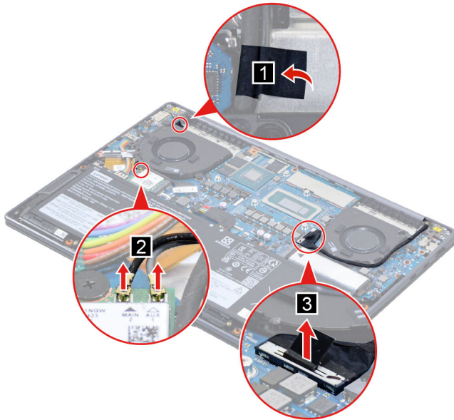
Figure 25. Disconnect the EDP cable and antenna cable
