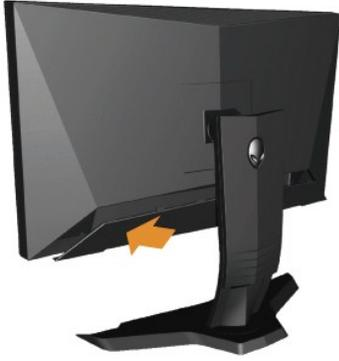
Attach the cable cover to the monitor after making the required cable connections to the monitor.
