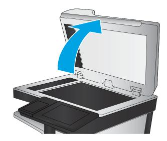
Clean the scanner glass, the document feeder strips, and the white plastic backing with a soft cloth or sponge that has been moistened with nonabrasive glass cleaner.
