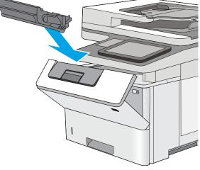
6. Align the toner cartridge with its slot, and then insert the toner cartridge into the printer.
