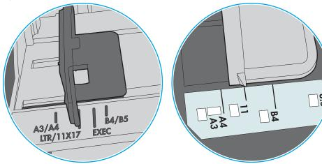
Figure 9-8 Size markings for Tray 1 or the multipurpose tray
