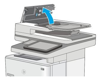
3. Remove any visible lint or dust from each of the feed rollers and the separation pad using compressed air or a clean lint-free cloth moistened with warm water.
