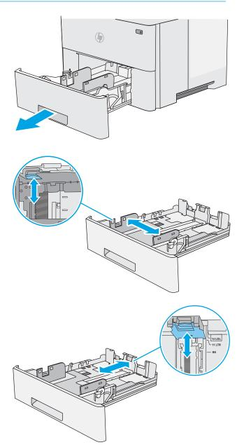
4. To load legal-size paper into the tray, squeeze the lever on the back of the tray that is to the left of center, and then extend the tray back to the correct paper size.
