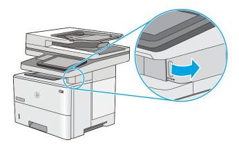
2. Remove the staple cartridge from the printer.
