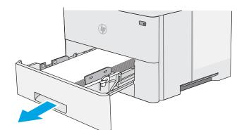
2. Pull forward on the green tab inside the tray area to release the duplex pan.
