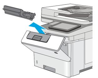
12. Lift the jam-access cover and slowly remove any jammed paper. Be careful not to tear the paper.
