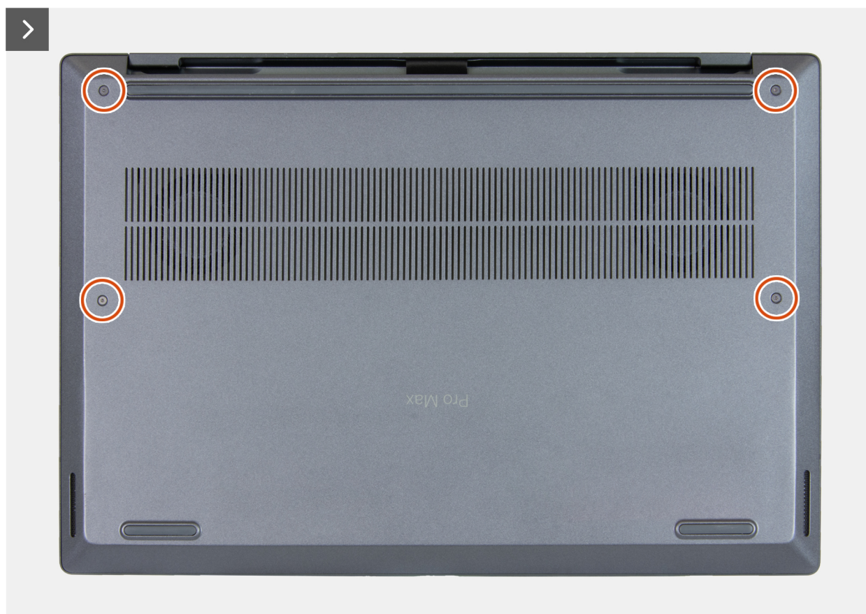
Figure 12. Removing the base cover
