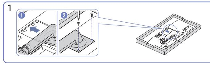
Push the stand neck into the main body in the direction of the arrow as shown in the figure. Tightly fasten the connecting screw on the bottom of the stand.
