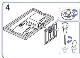
Insert the stand base into the stand in the direction of the arrow. Fasten the screw tightly (using a screwdriver or coin) into the bottom of the stand base.
