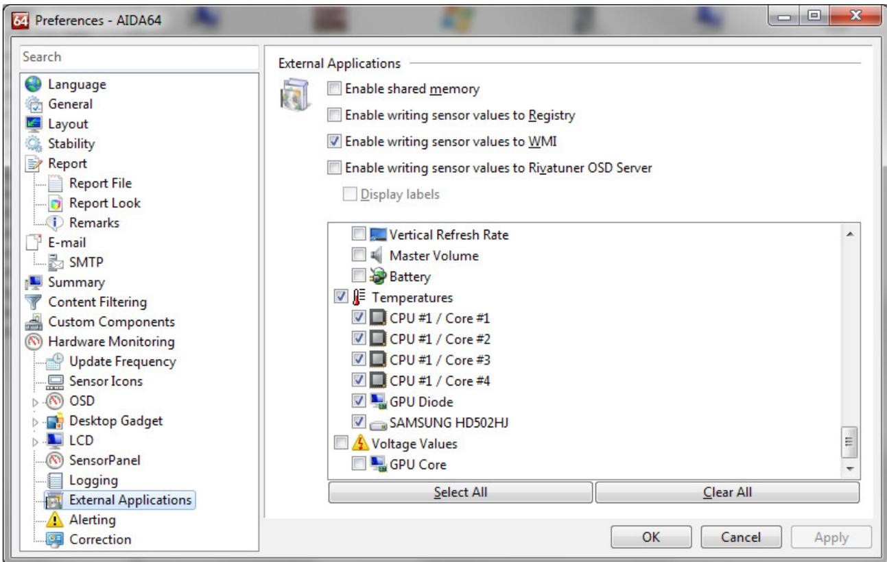
Click the "Select data source" button to assign each software sensor to a temperature sensor provided by third party software.
