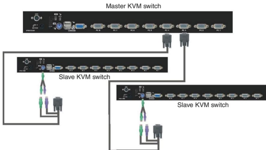
The maximum number of computers controlled by a Master/Slave configuration with all 8-port units is 64, with 8 Slaves and each Slave connecting to 8 computers:
