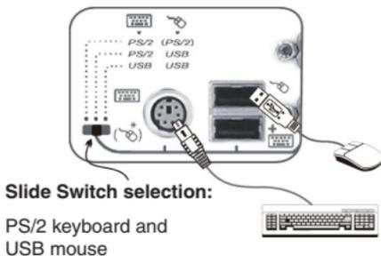
**USB Keyboard and USB Mouse:** Slide switch to the far right position.
