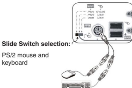
**PS/2 Keyboard and USB Mouse:** Slide switch to the center position
