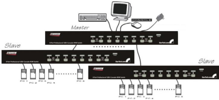
The maximum number of computers controlled in a Master/Slave configuration with all 16-port units is 136, with 8 units of 16-port Slaves (to PC 1 - PC 8) and each Slave connected to 16 computers, plus 8 more computers connected directly to the Master (to ports PC A - PC H):
