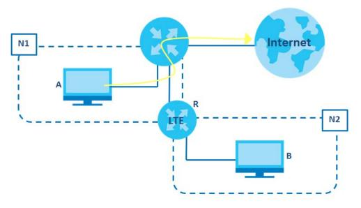
You need to specify a static routing rule on the LTE7460-M608 to specify **R** as the router in charge of forwarding traffic to **N2**. In this case, the LTE7460-M608 routes traffic from **A** to **R** and then **R** routes the traffic to **B**.
