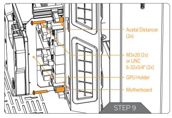
Use three or more screws to attach the GPU Holder to the left side of the PC case.
