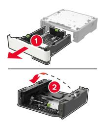
Remove the used pick roller assembly.
