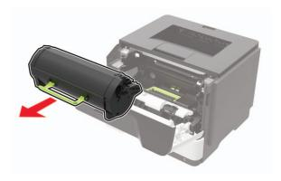
**3** Remove the used imaging unit.
