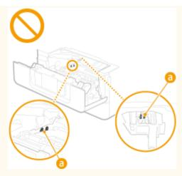
• To prevent a paper jam, do not turn OFF the power, open/close the covers, and load/unload the paper when printing.
