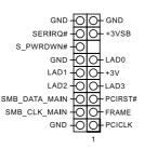
This connector supports Trusted Platform Module (TPM) system, which can securely store keys, digital certificates, passwords, and data. A TPM system also helps enhance network security, protects digital identities, and ensures platform integrity.
