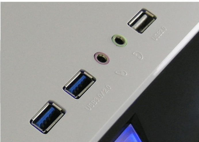
- I/O-Panel mit: 2x USB 3.0-Port; 1x USB 2.0-Port; HD Audio
