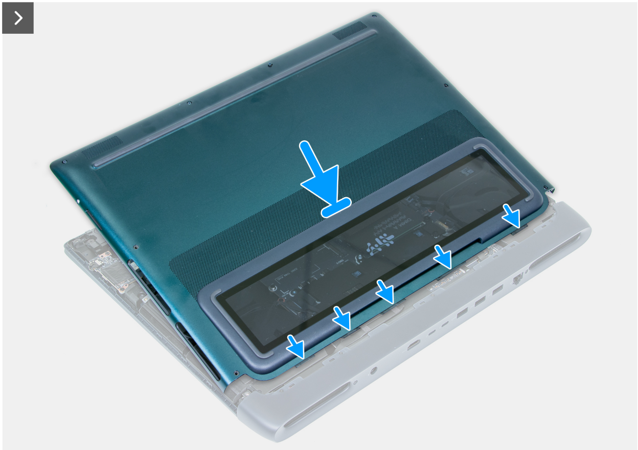
Figure 14. Slide the base cover
