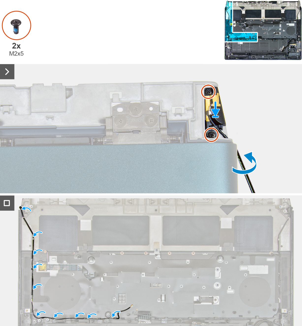
Figure 79. Installing the WLAN aux antenna
