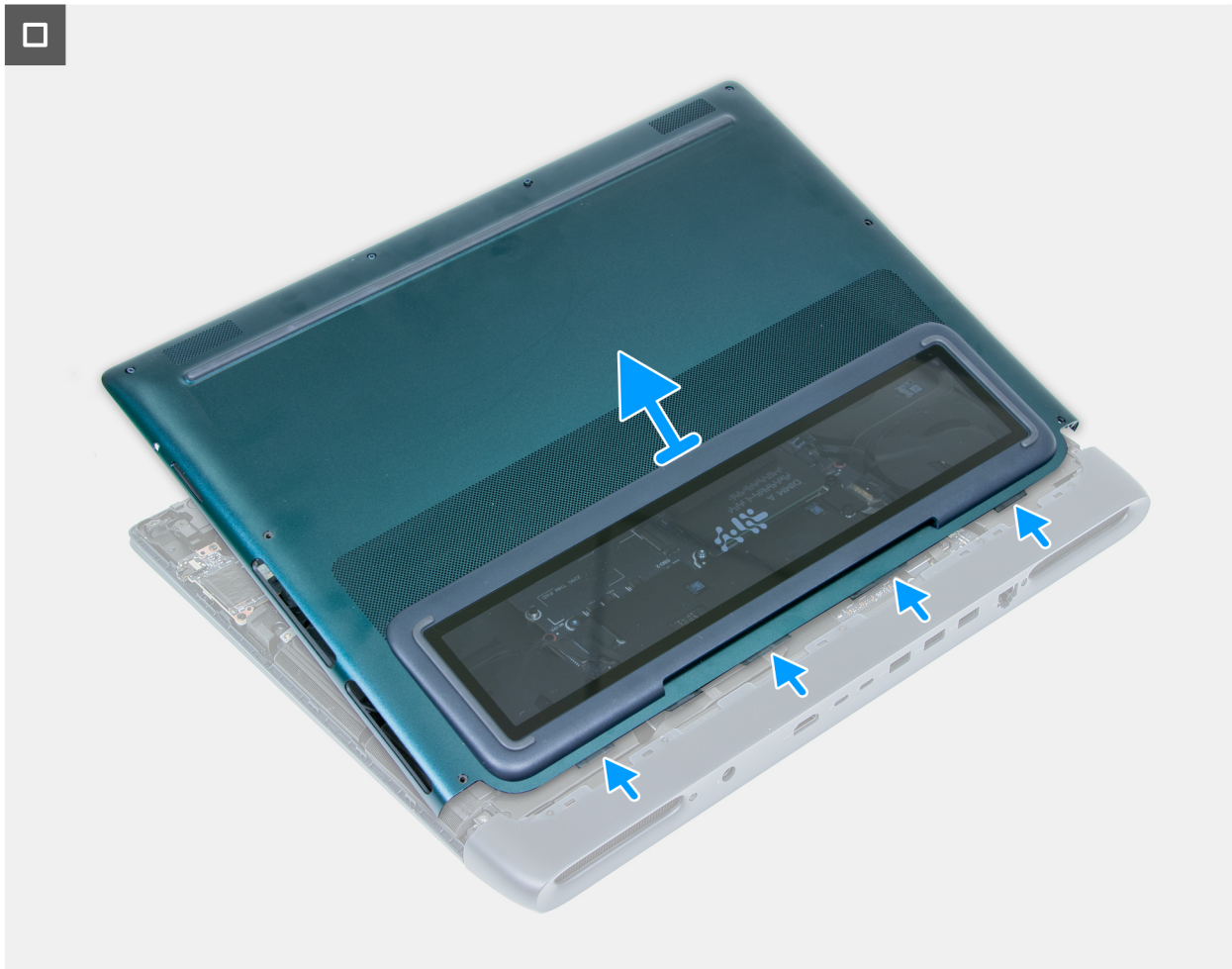
Figure 11. Lifting the base cover
