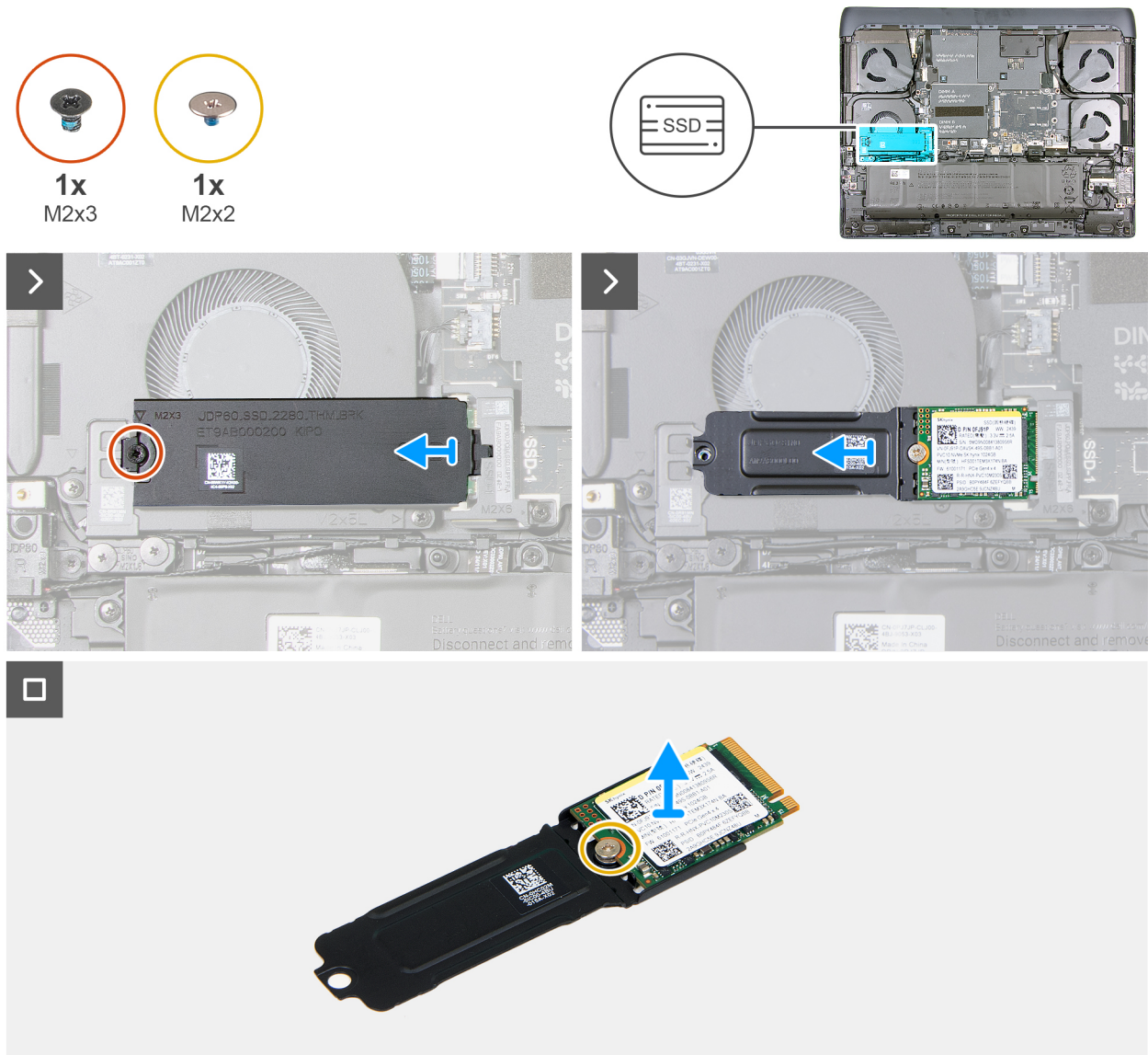
Figure 23. Removing the M.2 2230 SSD in slot 1
