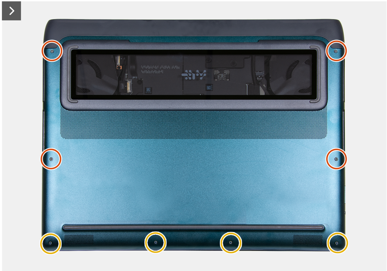
Figure 9. Removing the base cover screw
