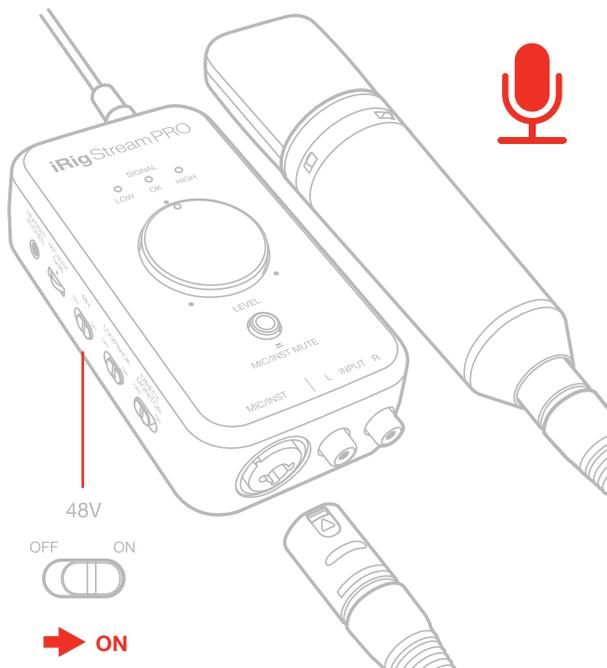
Before connecting a ribbon microphone, turn OFF phantom power and check the microphone's operating instruction manual to see if it requires it. Most ribbon microphones don't require phantom power, and some can even be damaged by it. If you're in doubt just leave it OFF. If the microphone won't work, check its user manual, it may need phantom power.
