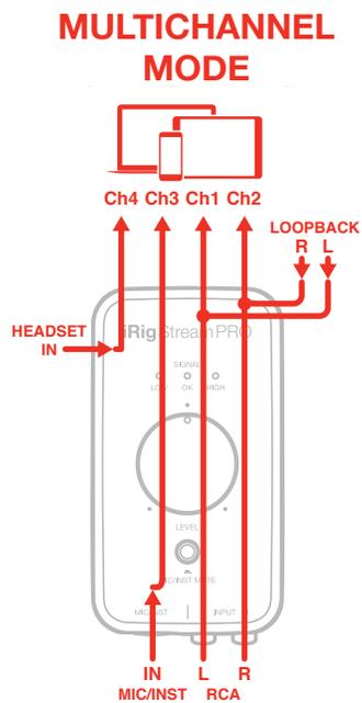
When the interface is set to multichannel mode, the “Mic/Inst Mute” button is lit green at low intensity.
