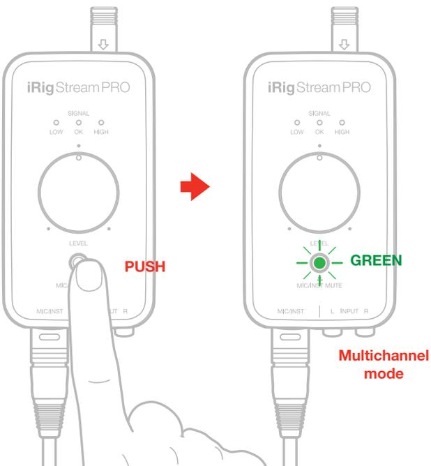
3. To confirm your selection, push and hold the “Mic/Inst Mute” button for 3 seconds. The button will remain lit green (low intensity) to indicate that you are currently in multichannel mode.
