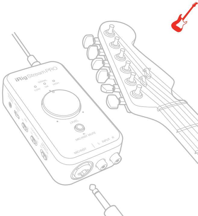
8. You can adjust the gain of the microphone/instrument input with the dedicate "Mic/Inst Gain" thumbwheel: if the level of the microphone/instrument input is too high the "Mute" button LED will light up RED for 2 seconds. You should decrease the gain. Also, you can control the post-gain level with the "Mic/Inst" level thumbwheel: this control helps you to adjust the level of the signal before the main Level knob.
