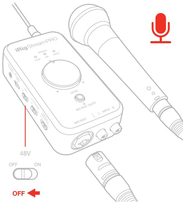
If you're using a condenser microphone, it will probably require external phantom power. If phantom power is ON, switch it OFF, and then connect your microphone. Turn phantom power ON only after the microphone is connected. If the "Mic/Inst Mute" LED flashes orange, check that working batteries are inserted in the iRig Stream Pro battery compartment on the bottom side, and that an application that is using iRig Stream Pro is open.
