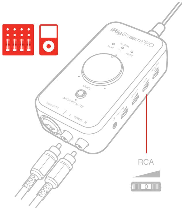
It is possible to connect any line level source to the RCA inputs. This signal can come from an mp3 player, a computer or an audio mixer. The main Level knob adjusts the overall volume that is recorded. To adjust the volume of the device connected to the RCA inputs, use both the volume controls of the device and the numbered thumbwheel “RCA” on the side of iRig Stream Pro.
