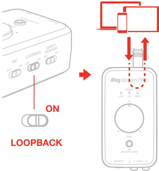
7. Now the processed signal from input 3 will come back to the inputs 1 and 2: these are the inputs usually used by your streaming app. You can control the level of the streamed signal by using the “Level” potentiometer.
