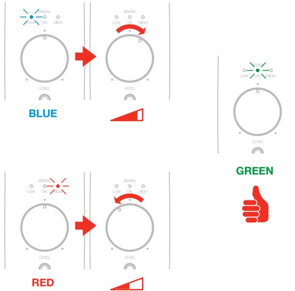
The three LEDs on iRig Stream Pro give you important information about the iRig Stream Pro's operating status. Each status is indicated by a different color:
