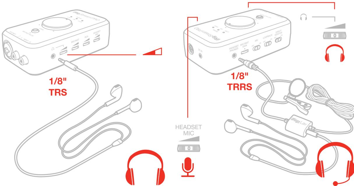
It is possible to connect an headset (compatible with CTIA wiring standard) or an iRig analogue microphone to the “Headset/Phones” port and an headphones to the “Headphones” port. The headset’s microphone gain can be controlled with the “Headset Mic” thumbwheel. In this case the main Level knob will control the overall signal level that is streamed to the connected host. If an headphones is connected, its volume can be controlled with the “Headphones” thumbwheel.
