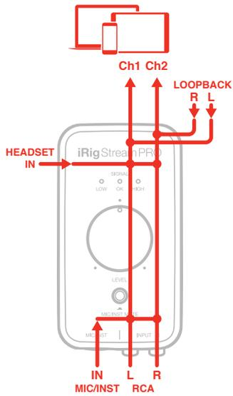
It is possible to change the configuration of the interface to multichannel mode, which will change the channel count as follows:
