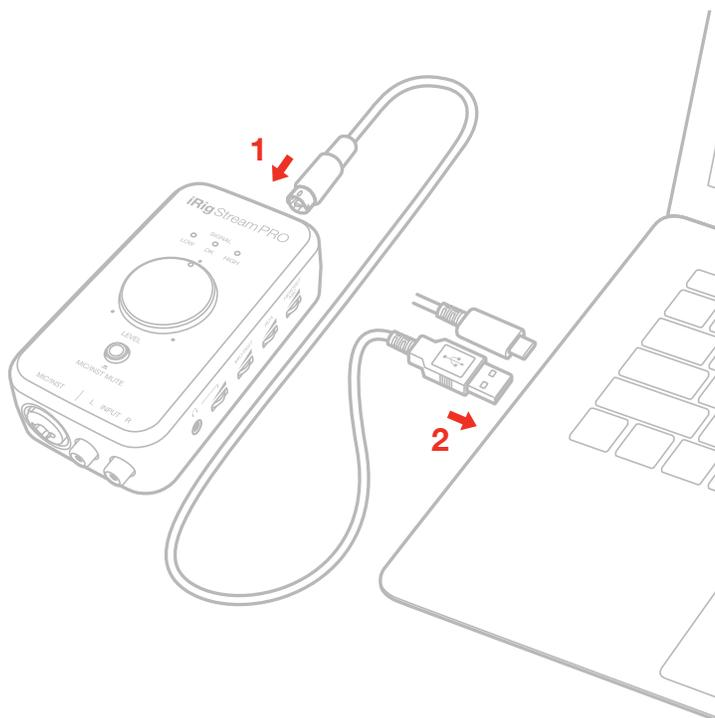
Once the iRig Stream Pro is connected to the host with the appropriate cable, launch your audio application and select iRig Stream Pro as the input/output device from your system's audio preferences. All the functionality described above allows you to cope with any registration and streaming needs.
