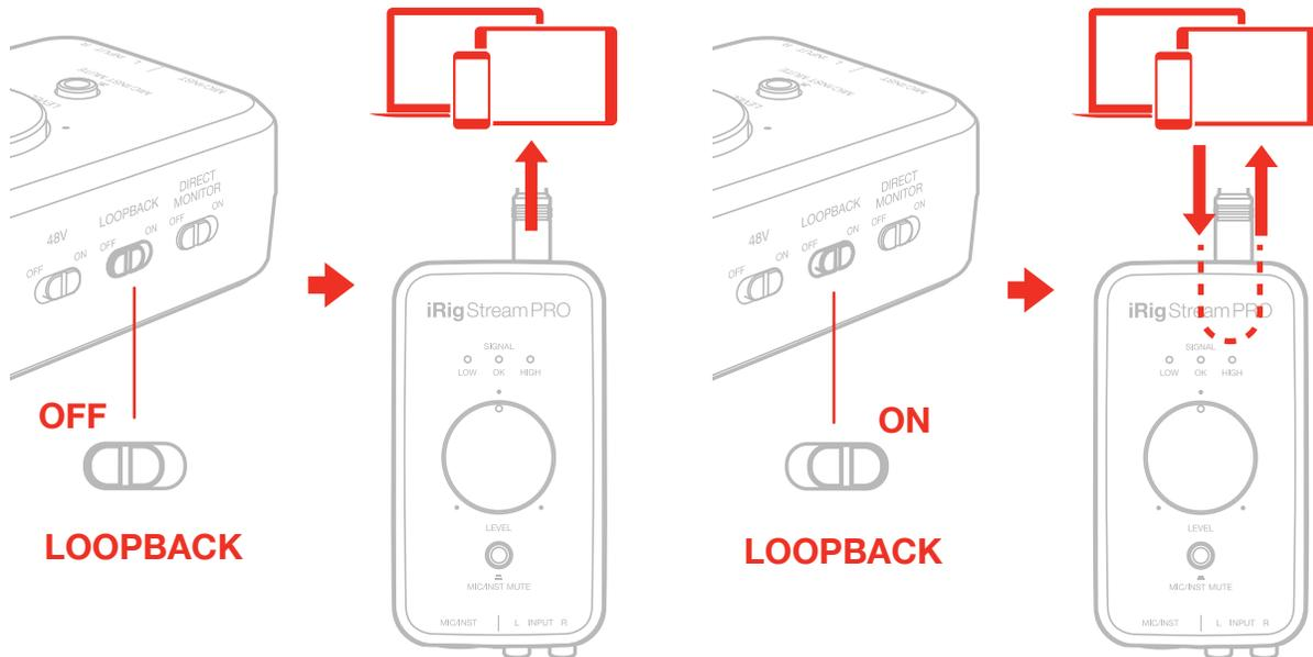
With the LOOPBACK function turned on, the audio that is input to the iRig Stream Pro from your host via USB is returned back to the host. The main Level knob will control the overall level that is recorded.
