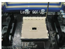
STEP 1: Lift Up The Socket Lever
