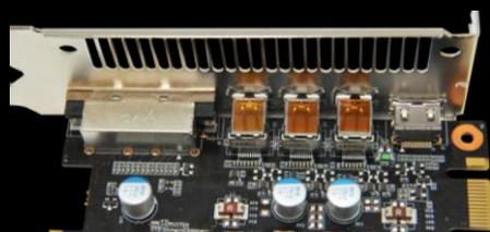
Five display ports located in a row, leave enough space on the top for the hot air to flow out
