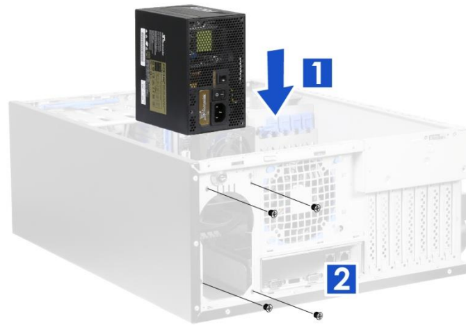
Figure 29 Single PSU installation
