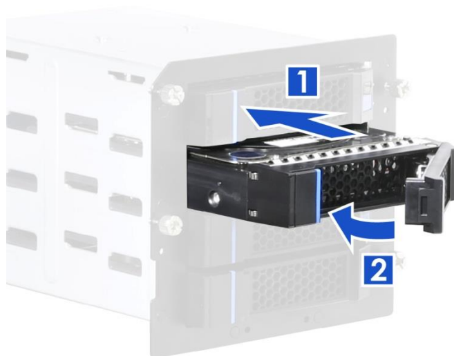
Figure 21 3.5" hot-swap HDD tray installation
