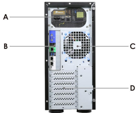
Figure 3 Back panel with redundant PSU
