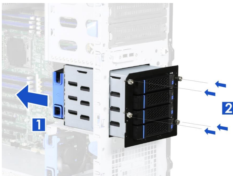
Figure 17 3.5" hot-swap HDD cage installation
