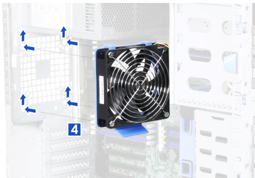
Figure 28 Rear fan maintenance step- 2
