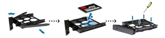
3 Insert the drive tray into the empty drive bay and push it back until you hear a click when the tray is locked into place.
