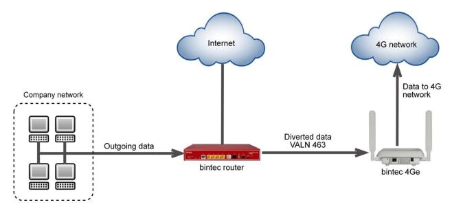
The **bintec 4Ge** operates in DHCP client mode. The configuration parameters are sent as ASCII values from the connected router using DHCP option 43. The **bintec 4Ge** can be operated on a PoE switch or connected directly to the Ethernet port of a router. The connected LAN must have an active DHCP server that can provide an ASCII value as option 43 (vendor-specific string).
