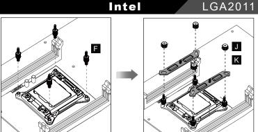
For LGA2011, screw the "Screw F" on the motherboard directly
