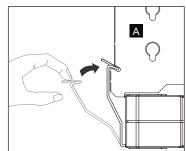
Attach the fan using the supplied steel clips for maximum cooling performance.
