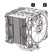
Forza 85 comes with an additional set of fan clips that allows for a second 120 mm fan of any brand to increase the heat dissipation efficiency of the Forza 85. To maximize the performance,we recommend a second COUGAR MHP 120 fan (sold separately).
