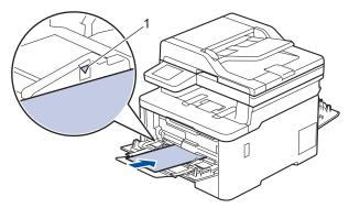
Load up to three envelopes in the MP tray with the printing surface face up. Make sure the envelopes are below the maximum paper mark (1). Loading more than three envelopes may cause paper jams.
