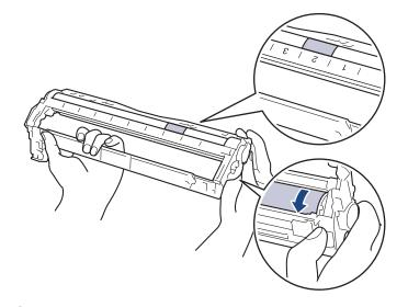
Use the column numbers next to the drum roller to find the mark. For example, a dot in column 2 on the Drum Dot Check Sheet would mean that there is a mark in the "2" region of the drum.
