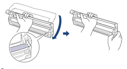
To avoid print quality problems, DO NOT touch any surface of the drum unit except the drum unit gear.
