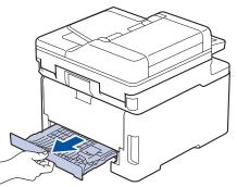
4. Pull the jammed paper out of the machine or out of the 2-sided tray.
