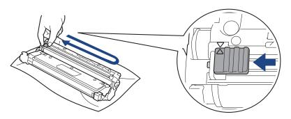
Be sure to return the green tab to the Home position (▲). The arrow on the tab must be aligned with the arrow on the drum unit. If it is not, printed pages may have a vertical stripe.
