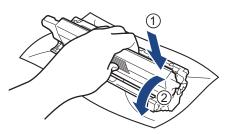
Make sure you put the toner cartridge in correctly or it may separate from the drum unit.
