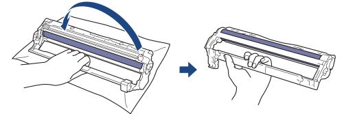
9. Loosen your grip so the frame drops forward, and then use your right hand to locate the drum unit gear inside the right side of the frame.
