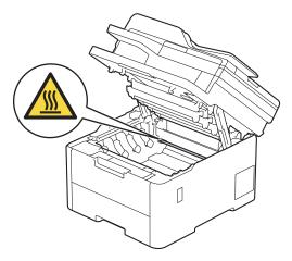
2. Remove the toner cartridge and drum unit assembly.
