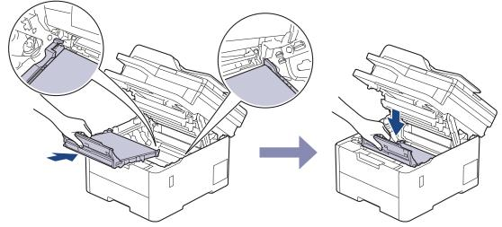
9. Reinsert each toner cartridge and drum unit assembly into the machine. Make sure that you match the toner cartridge colour to the same colour label on the machine for all four toner cartridge and drum unit assemblies.
