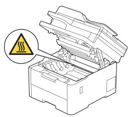
6. The colour of printed dots on the Drum Dot Check Sheet is the colour of the drum you should clean. Remove the toner cartridge and drum unit assembly that matches the colour causing the problem.
