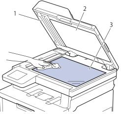
3. In the ADF unit, clean the white bar (1) and the scanner glass strip (2) underneath it with a soft lint-free cloth moistened with water.
