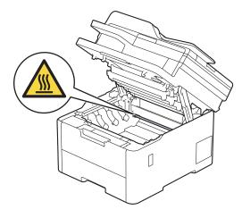
3. Remove the toner cartridge and drum unit assembly for the colour shown on the LCD.
