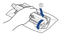
Make sure you put the toner cartridge in correctly or it may separate from the drum unit.
