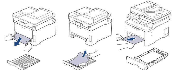
5. Remove paper that may have jammed under the machine due to static electricity.
