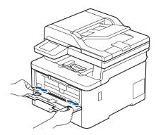
4. Using both hands, place one sheet of paper in the manual feed slot until the front edge touches the paper feed roller. When you feel the machine pull it in, let go.
