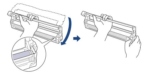
To avoid print quality problems, DO NOT touch any surface of the drum unit except the drum unit gear.
