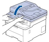
• You can still use the machine while the scanner cover is up. To close the scanner cover, gently push it down with both hands.
