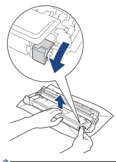
Jo avoid print quality problems, DO NOT touch any surface of the drum unit except the drum unit gear.
