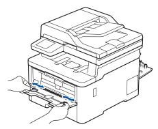
5. Using both hands, put one envelope in the manual feed slot until the front edge touches the paper feed roller. When you feel the machine pull it in, let go.
