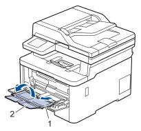
4. Slide the MP tray paper guides to fit the width of the paper you are using.
