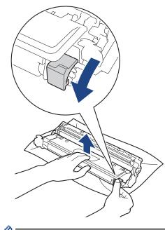
To avoid print quality problems, DO NOT touch any surface of the drum unit except the drum unit gear.
