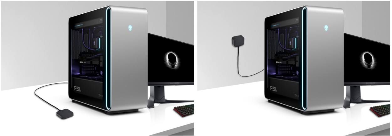
Figure 14. Placing the antenna in a suitable location
