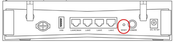
Figure 13 Reset Button (LTE7240-M403)
