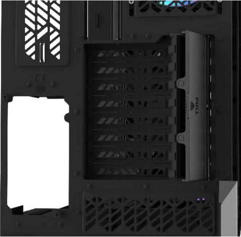
**Tool-less Vertical GPU Mounting (Patent Pending)**
