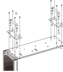
1. Remove L-shaped handle bar brackets on both sides
