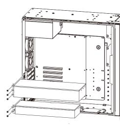
4. Install 3 x 2.5" SSD on the expansion card retainer
