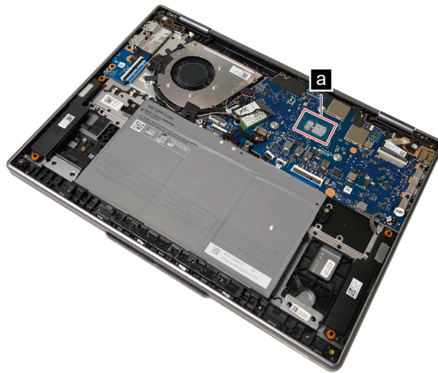
Figure 3. Area(s) on the system board where thermal interface materials are applied
