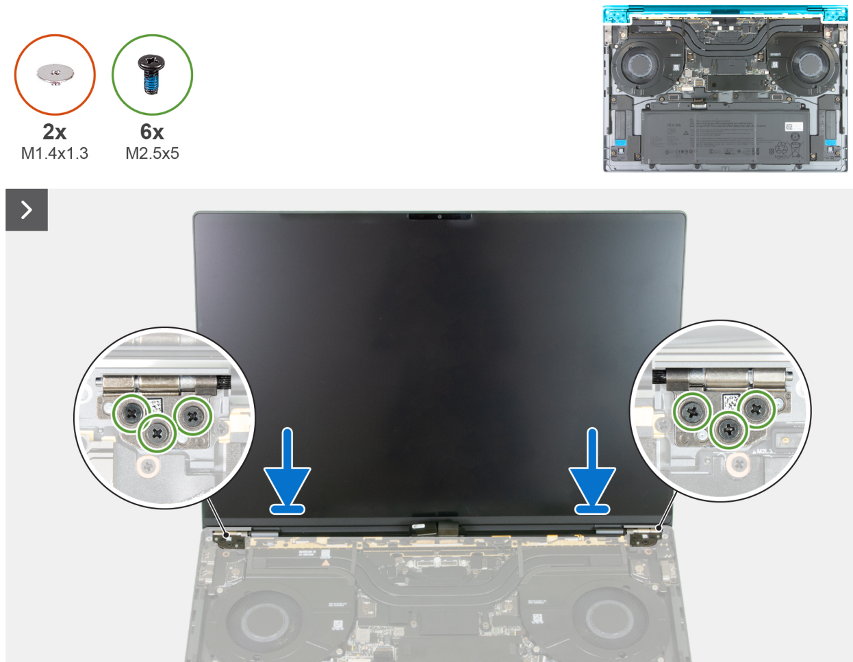
Figure 19. Installing the display assembly
