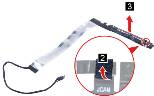
Figure 37. Remove the tape and remove the camera
