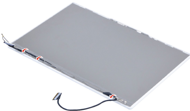
Figure 28. Release the EDP cable and camera cable from the cable guide
