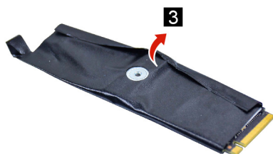
Figure 8. Remove the SSD mylar
