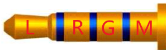
Figure 17 Definition of four-segment headphones
