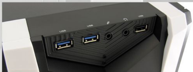
- I/O-Panel with: 2x USB 3.0 port, 1x USB 2.0 port, HD Audio
