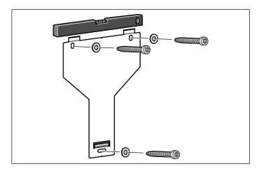
Screw in the mounting supports for the extractor hood until they are hand-tight, use a spirit level to level the appliance and then screw the mounting supports in fully.
