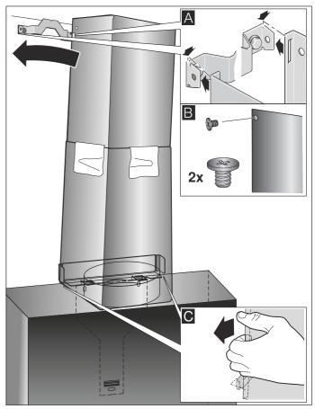
7. Clip the lower flue duct section in at the retaining bracket. The connection cable must not be damaged.
