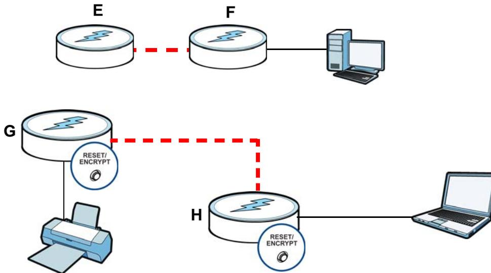
If the HomePlug (🏠) lights on both powerline devices do not light up, the powerline devices are not connected. Repeat the connection process, making certain you press the **RESET/ENCRYPT** buttons for the correct time and within two minutes of each other. If that does not work see Section 6.4 on page 48 for suggestions.
