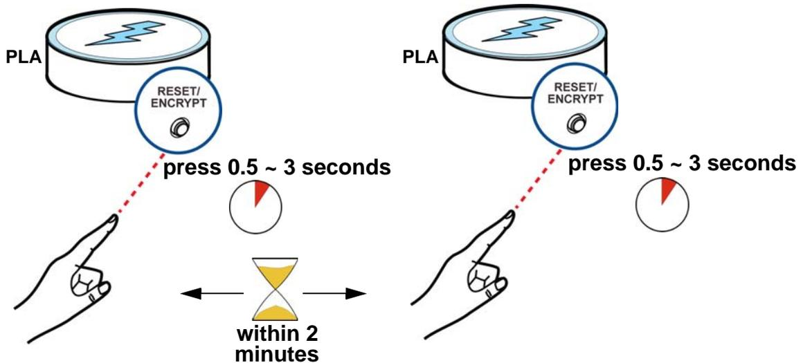
Note: The **RESET/ENCRYPT** button's location varies for each Powerline model.
