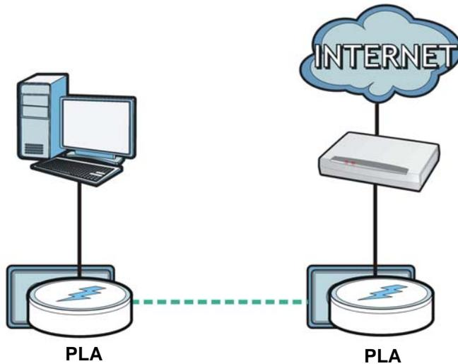
Connect your PLA to an Internet gateway such as a modem and plug it into an ordinary power outlet in your home. Plug a second PLA into another power outlet and connect a computer to the PLA for Internet access. Your network can be further expanded by plugging additional PLAs into other outlets in your home and connecting other computers or network devices (for example, a printer) to them.
