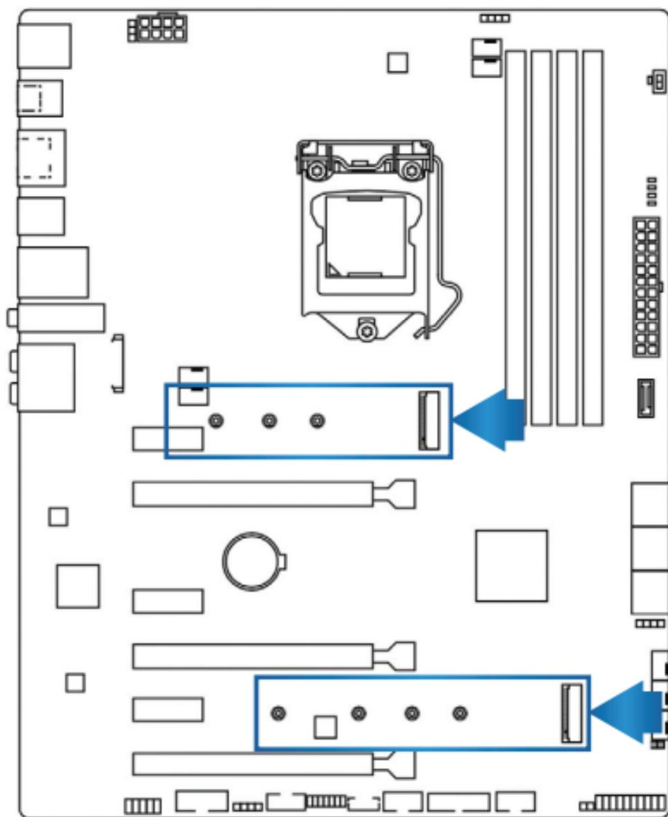
8. Insert the **Sabrent ROCKET Q NVMe M.2 SSD** device pin-side first into the M.2 slot as is illustrated below.
