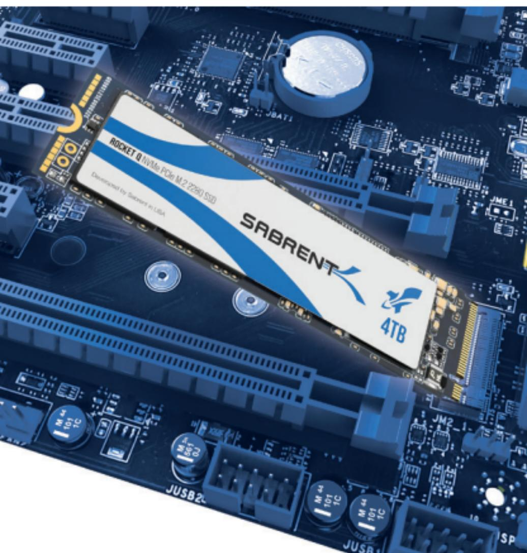
9. Fasten the opposite end of the **Sabrent ROCKET Q NVMe M.2 SSD** to the motherboard with the necessary screw or hardware, as is illustrated below.
