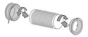
2. Connect the suitable end of the exhaust air hose to the exhaust air hose connection (7) located at the device.
