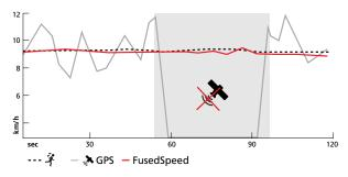
FusedSpeed benefits you the most when you need highly reactive speed readings during training, for example, when running on uneven terrain or during interval training. If you temporarily lose the GPS signal, for example, Suunto Ambit3 Run is able to continue showing accurate speed readings with the help of the GPS calibrated accelerometer.
