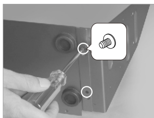
Use "H" screw to secure bottom panel on the right panel
