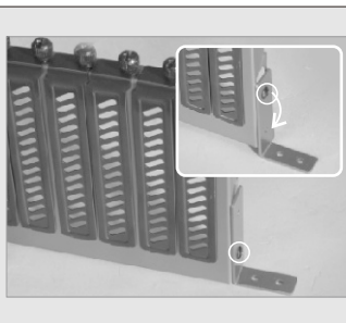
Secure the PCI slots bracket on the M/B tray with "D" screw 6pcs
