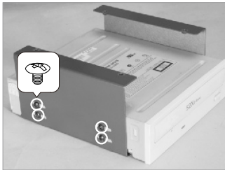
Use "D" screw to secure CD-ROM support bracket on the CD-ROM
