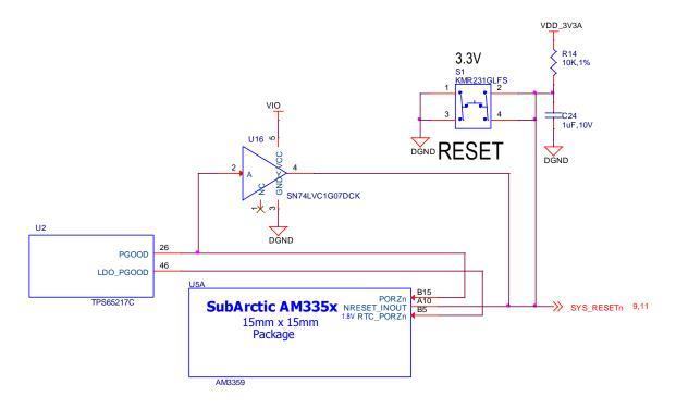
Figure 31. Board Reset Circuitry
