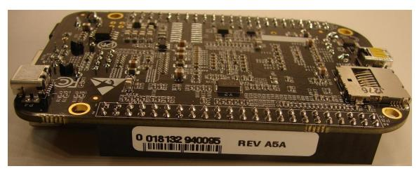
Figure 78. Third Phase Serial Number and Revision Location
