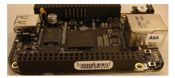
Figure 77. Second Phase Serial Number and Revision Location
