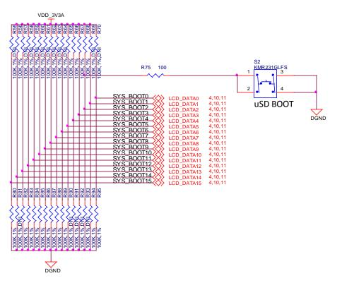
Figure 38. Processor Boot Configuration Design
