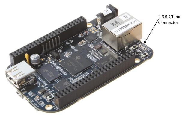
Figure 52. USB Client Connector
