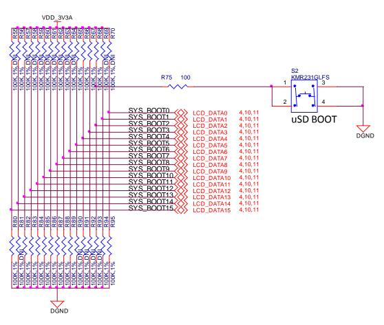
Figure 63. Expansion Boot Pins
