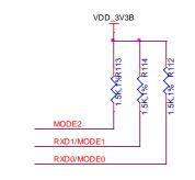
Figure 43. Ethernet PHY Mode Pins
