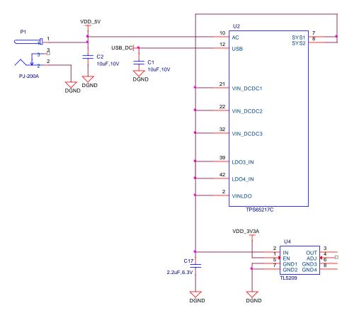
Figure 23 below shows how the DC input is connected to the TPS65217C.
