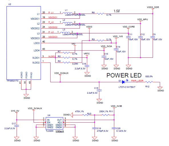
Figure 25 shows the connections of each of the rails from the TPS65217C.
