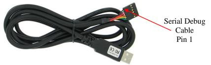
Figure 55. FTDI USB to Serial Adapter
