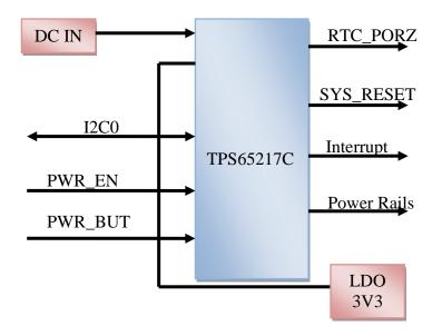
Figure 21. High Level Power Block Diagram
