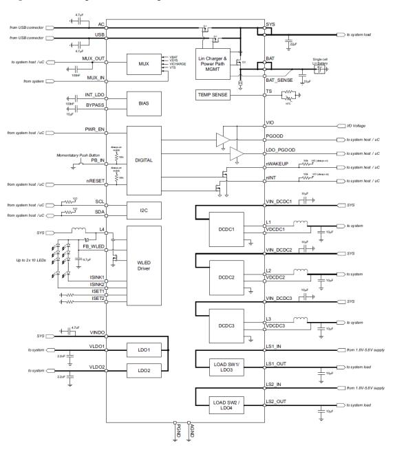
Figure 22 is the high level block diagram of the TPS65217C.
