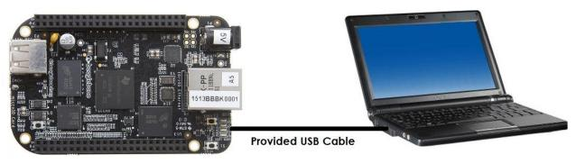
Figure 2. Tethered Configuration
