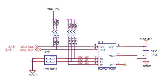
Figure 61. Expansion Board EEPROM Without Write Protect
