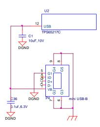
Figure 24. USB Power Connections
