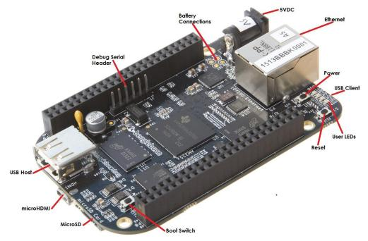
Figure 17. Connectors, LEDs and Switches
