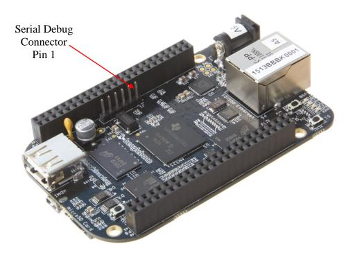
Figure 54. Serial Debug Header
