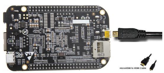
Figure 14. Connect microHDMI Cable to the Board
