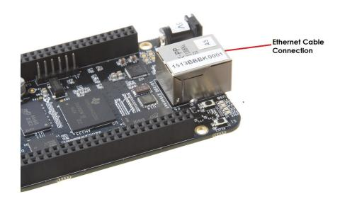
Figure 12. Ethernet Cable Connection
