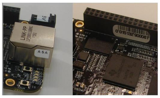
Figure 76. Initial Serial Number and Revision Locations
