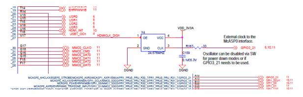
Figure 45. 24.576MHZ Oscillator
