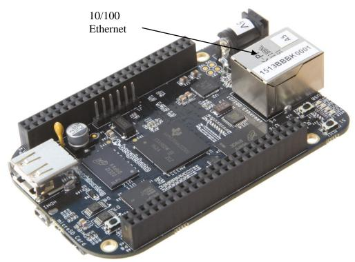
Figure 60. Ethernet Connector
