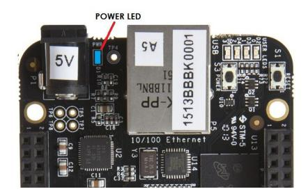
Figure 4. Board Power LED
