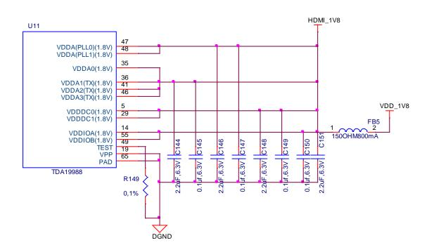
Figure 46. HDMI Power Connections
