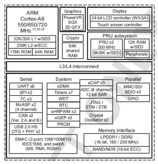
Figure 29. Sitara AM3358BZCZ Block Diagram
