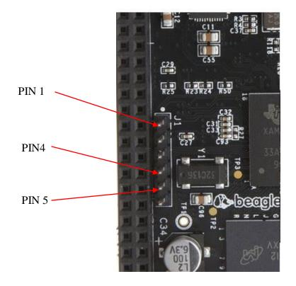
Figure 56. Serial Header
