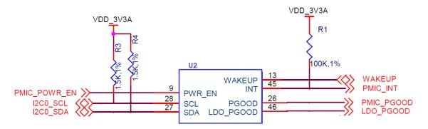
Figure 28. Power Processor Interfaces
