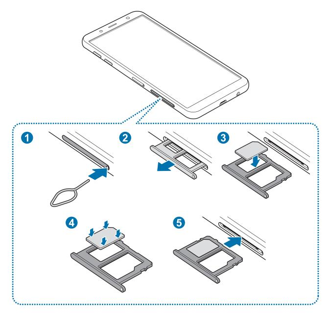
1 Insert the ejection pin into the hole on the tray to loosen the tray.
