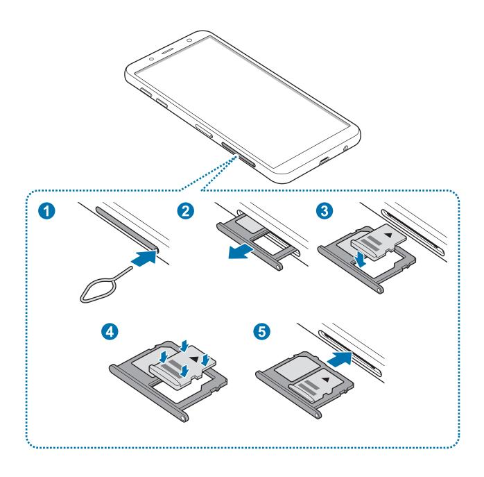
1 Insert the ejection pin into the hole on the tray to loosen the tray.
