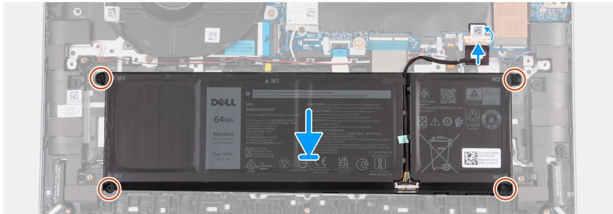
Figure 22. Installing the 4-cell battery (64 Wh)
