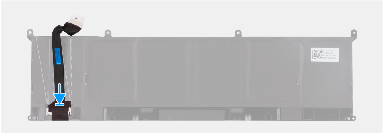
Figure 28. Installing the 90 Wh battery cable
