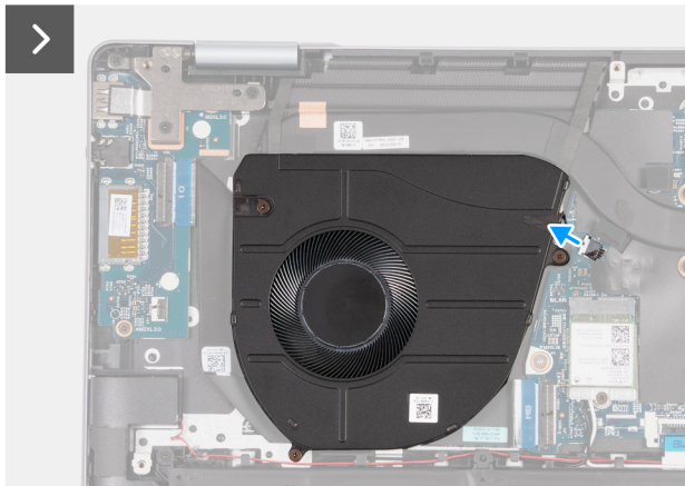
Figure 17. Removing the fan
