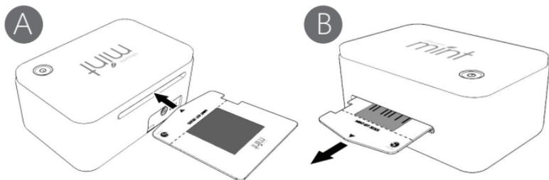
*NOTE: If the sheet holder catches on something inside or is not ejected correctly, slide the release lever on the bottom of the Mint towards the **RELEASE** side and then pull out the stamp sheet. Next, return the release lever to the **PRINT** side and perform printing again. If you experience problems using the same sheet holder, use a new one.*
