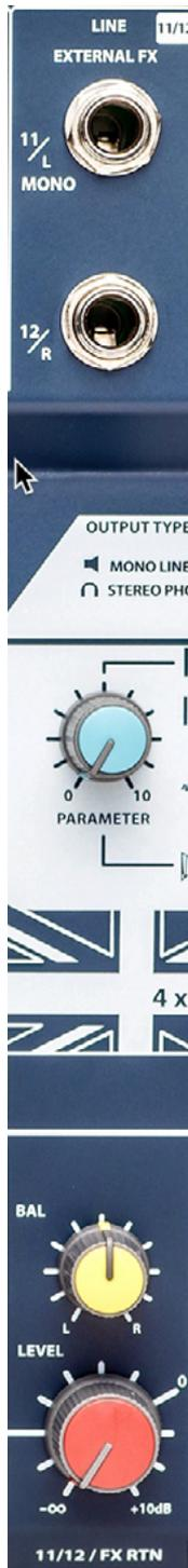
Aux/FX send is pre-fade due to the dual use of the Aux bus. An input channel's contribution to that Aux Send processing field is independent to that channel's Level contribution to the main stereo mix.
