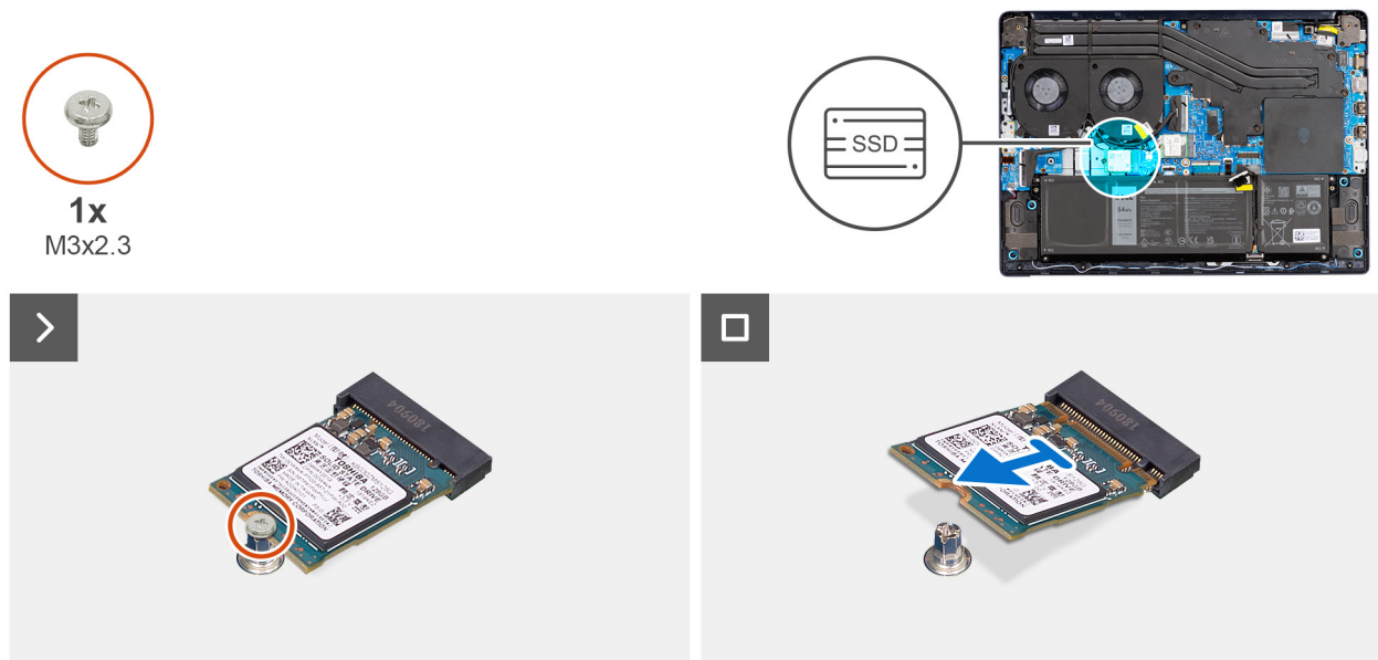
Figure 14. Removing the M.2 2230 SSD
