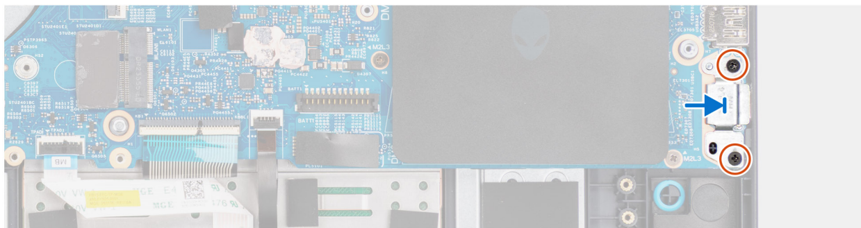
Figure 26. Installing the USB Type-C bracket (system board)
