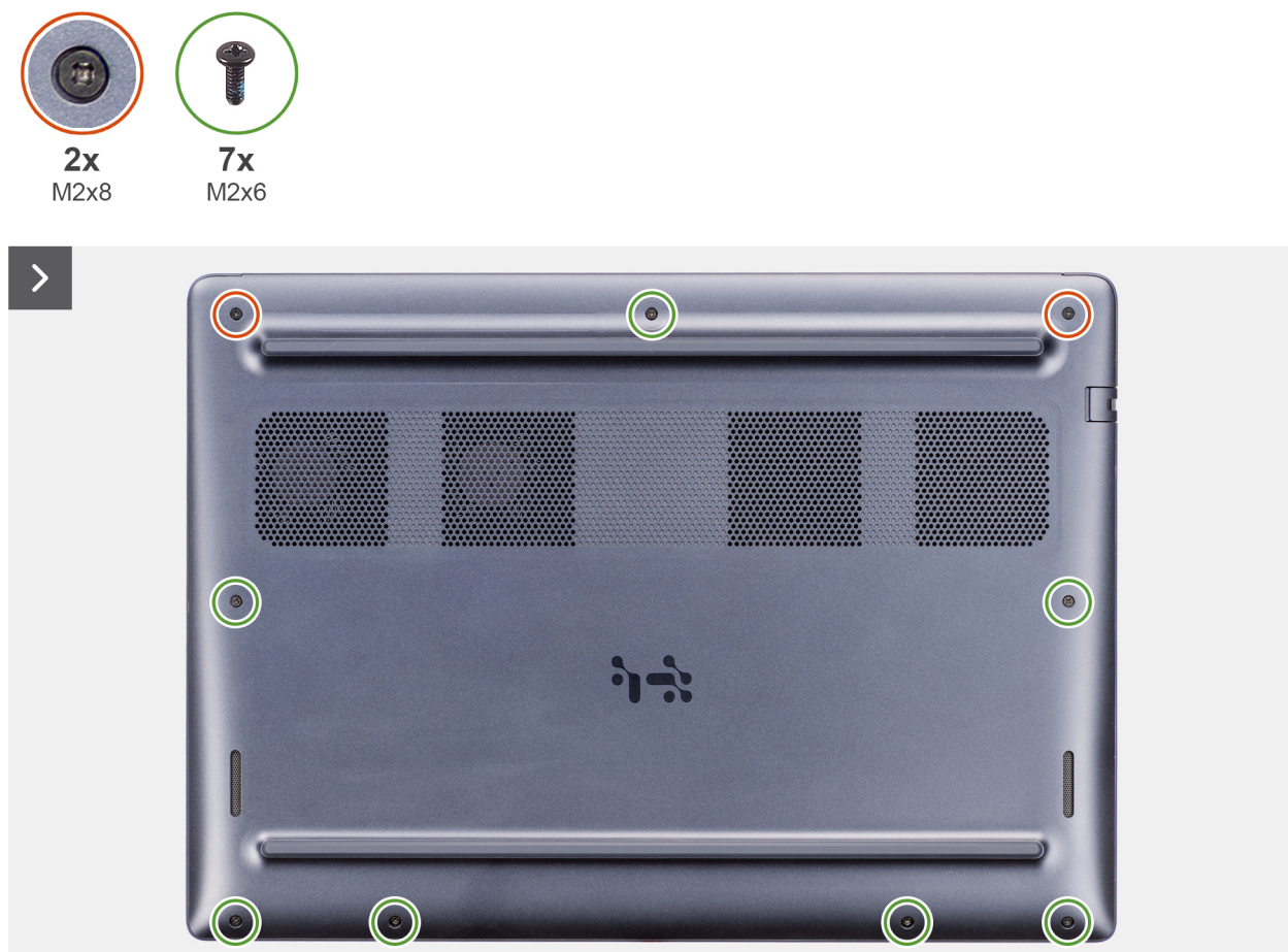
Figure 2. Removing the base cover
