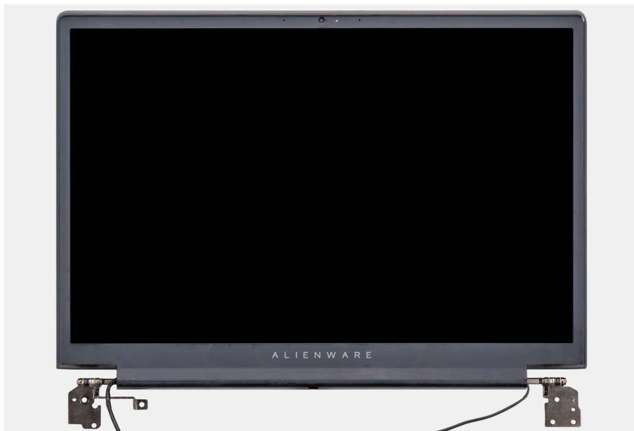
Figure 49. Installing the display assembly
