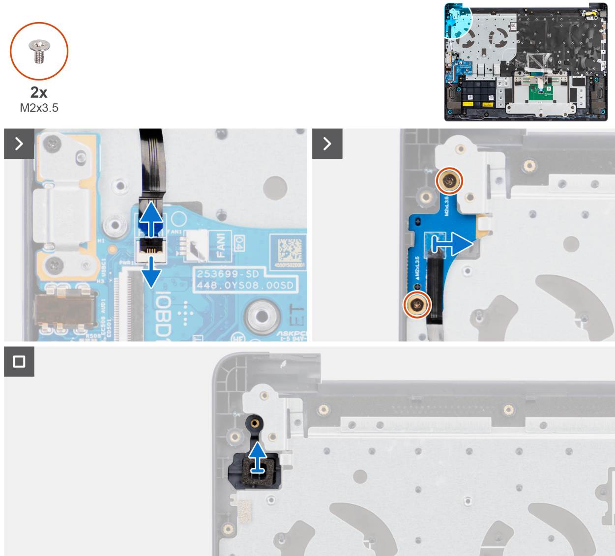
Figure 53. Removing the power button and power-button board
