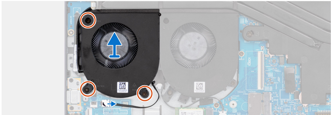
Figure 31. Removing the left fan
