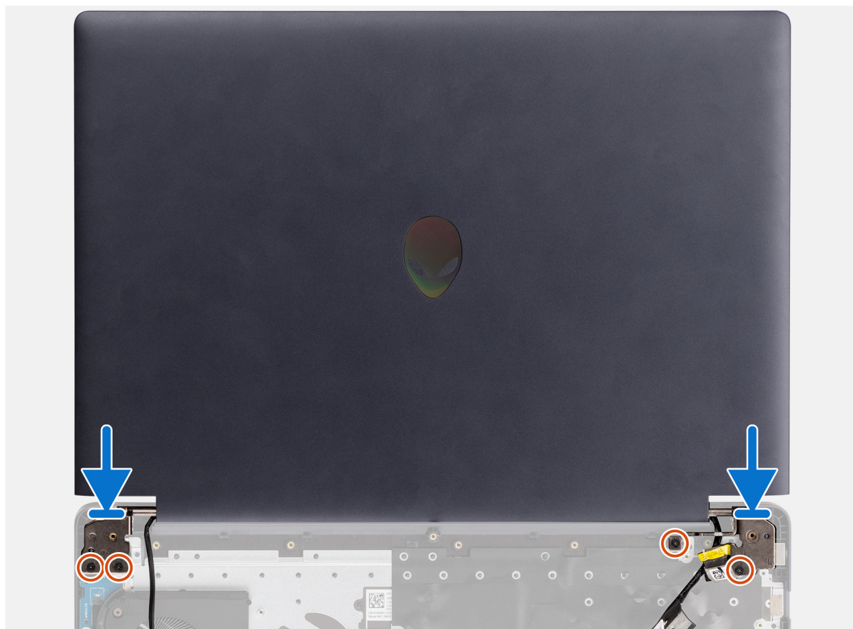
Figure 50. Installing the display assembly
