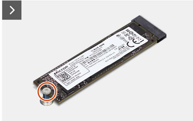
Figure 16. Removing the M.2 2280 SSD
