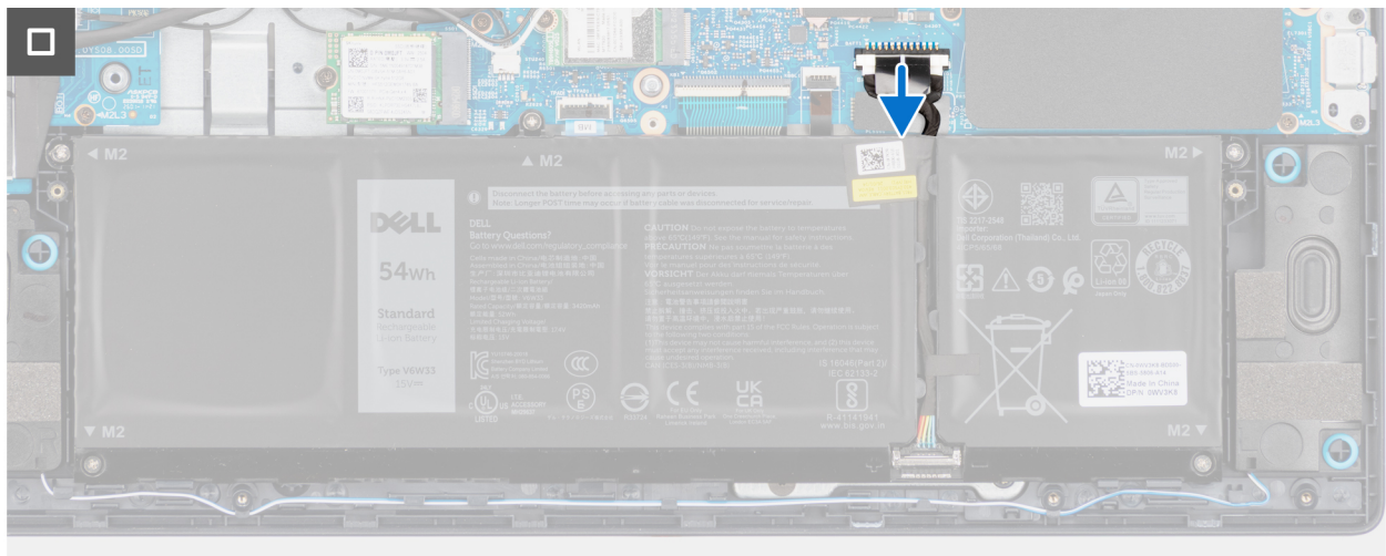
Figure 4. Disconnecting the battery cable
