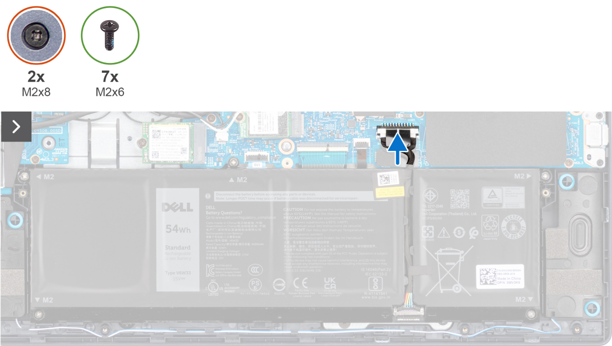
Figure 5. Connecting the battery cable
