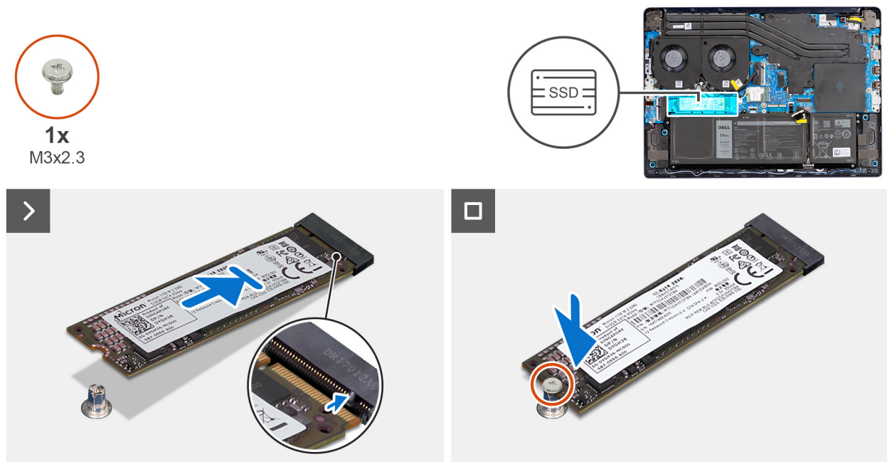
Figure 17. Installing the M.2 2280 SSD
