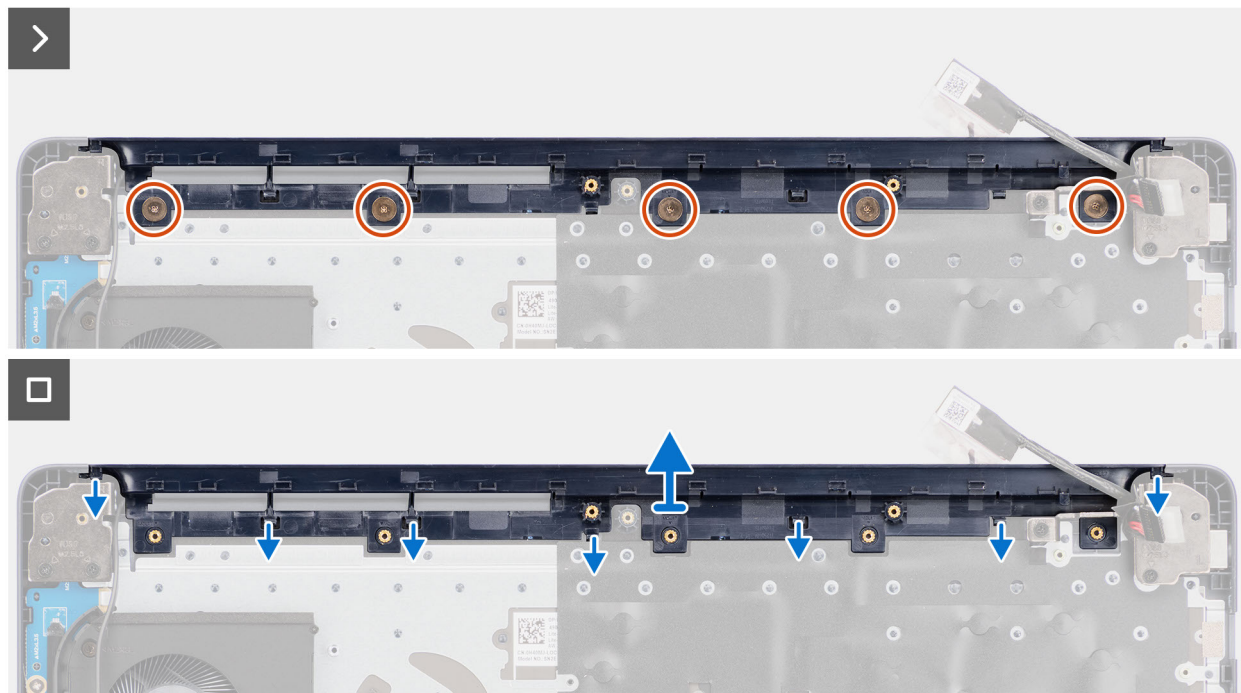
Figure 45. Removing the deco cover
