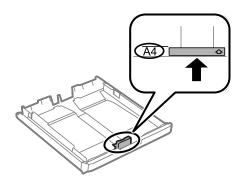
5. With the printable side facing down, load paper against the front edge guide.
