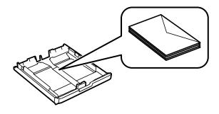
☐ Fan and align the edges of the envelopes before loading. When the stacked envelopes are puffed up with air, press them down to flatten them before loading.
