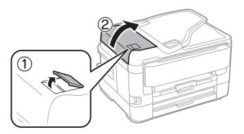
2. Use a soft, moist cloth to clean the roller and the interior of the ADF.
