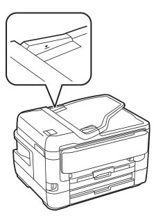
☐ Check that the ADF icon is on at the bottom of the screen. If it is off, place the originals again.
