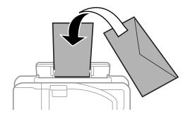
Load envelopes in the paper cassette with the flap facing up, and then slide the edge guides to the edges of the envelopes.
