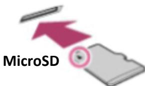
3. Place the memory card into the correct section of the tray, with the proper orientation. When inserting the Micro SD card, make sure the metallic contacts face down. Insert the card until it clicks and locks into place. To release the card, push and release it, then pull it out.
