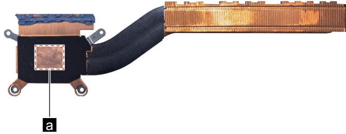
Figure 11. Areas on the heat sink where thermal interface materials should be applied
