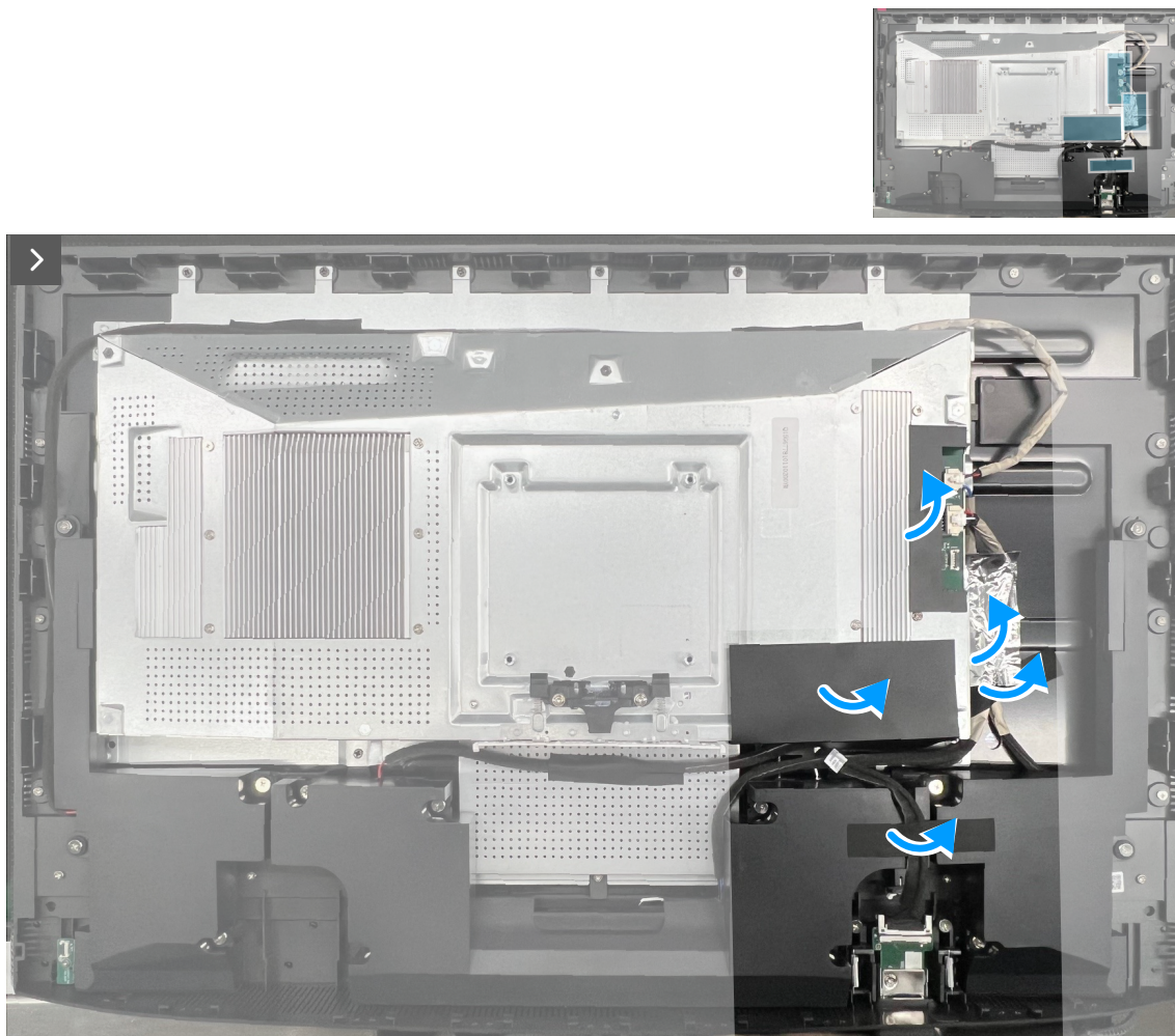
Figure 19. Peeling the tapes to secure the cables and Mylar
