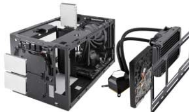
120mm radiator at the rear, 120mm radiator on the side 3.5" HDD x 1 + 2.5" SSD x 3
