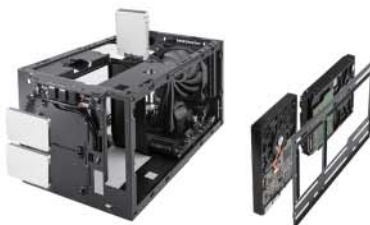
120mm radiator at the rear, 120mm radiator on the side 3.5" HDD x 1 + 2.5" SSD x 3
