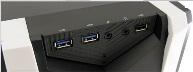
- I/O-Panel mit: 2x USB 3.0-Port, 1x USB 2.0-Port, HD Audio
