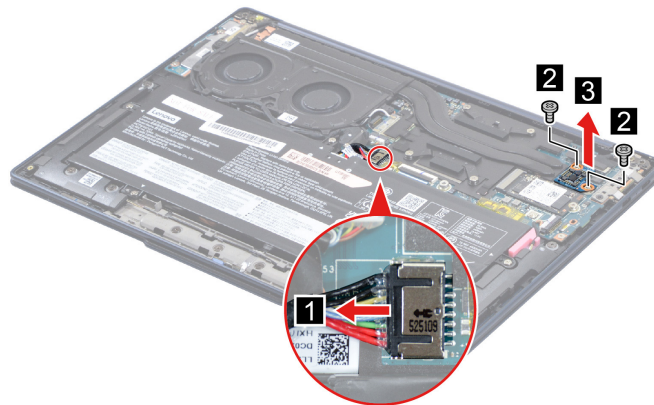
Figure 15. Remove two screws and remove the PMIC board
